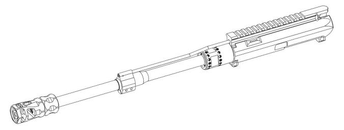
6) Slide the rail over the barrel, gas block and tube all the way to the upper receiver and verify that the barrel nut is in the correct position
