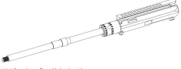
4) Install your low profile gas block and gas tube
