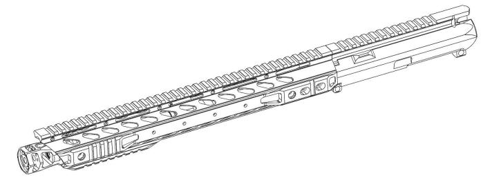
7) Loosely install the six socket head cap screws. If your rail has two screw types, the low-profile cap screws will go in the 6 o'clock position. The low head cap screws use a 3/32" Allen wrench, and the standard socket head cap screws use a 5/32" Allen wrench.
