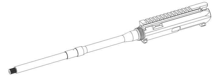
2) Apply a small amount of anti-seize lubricant to the upper receiver threads to protect them.
